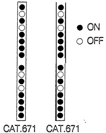
If the reading on the oscilloscope is similar to the above one, with a not correct reading of the data on the CAT. 671, you have to move the CCD board towards the operator after having loosened the “K” screws.
